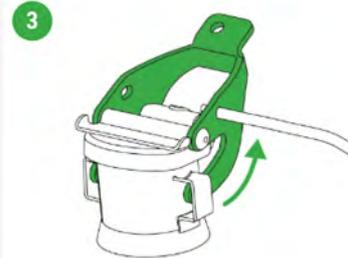
Lift the lever until the arms are fully released from the holder.
