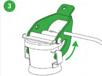
3 Lift the lever until the arms are fully released from the holder.
