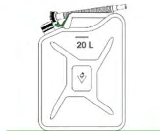
If the fuel can is equipped with a fuel spout holder, attach the spout to the holder for easier transportation.
