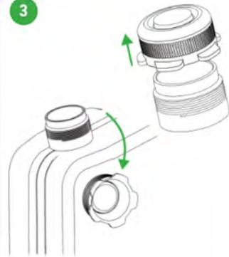
Place the removed cap on the fuel can with the help of the incorporated magnet.
