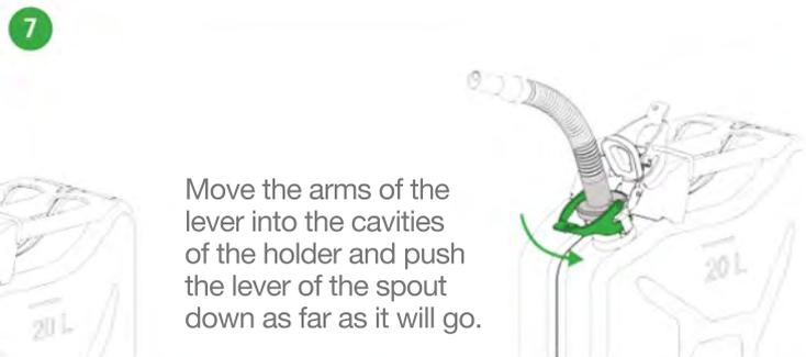
7 Move the arms of the lever into the cavities of the holder and push the lever of the spout down as far as it will go.
