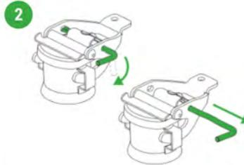
Turn the locking pin and pull it out of the lever as far as it will go.
