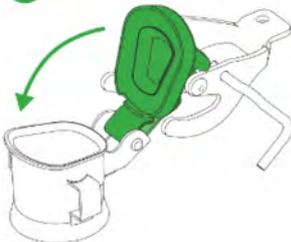
Push the lever forward until the lid completely covers the neck opening.
