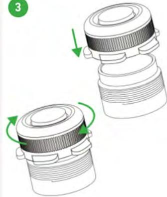
Place the cap back on the neck of the fuel can. Close the fuel can shut by screwing the cap clockwise.
