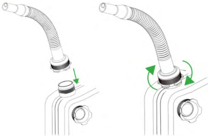
Screw the spout on by turning it clockwise until you feel resistance of the seal. Then turn the spout an additional 1/4 of a turn.
