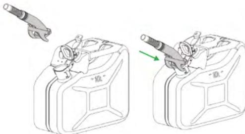
By pulling the lever, lift the lid up to open the neck opening.
