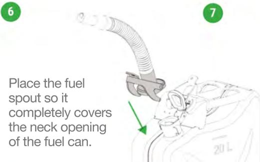
6 Place the fuel spout so it completely covers the neck opening of the fuel can.
