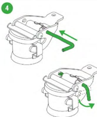
Insert the locking pin through the lever and rotate in 90degrees.
