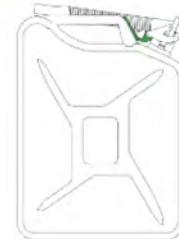
If the fuel can is equipped with a spout holder, attach the spout to the holder for easier transportation.
