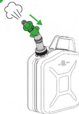
Before filling the fuel, press the tip of the spout to even out the fuel vapour pressure in the fuel can.
