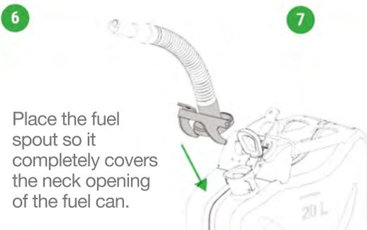
Place the fuel spout so it completely covers the neck opening of the fuel can.
