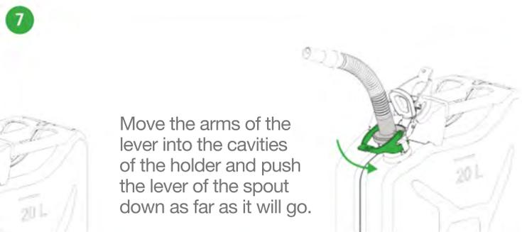
Move the arms of the lever into the cavities of the holder and push the lever of the spout down as far as it will go.
