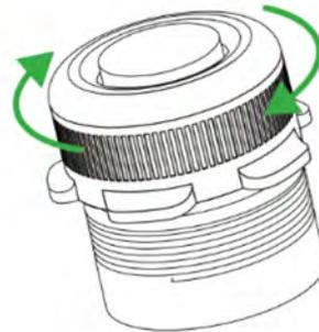
Close the fuel can shut by screwing the cap clockwise.
