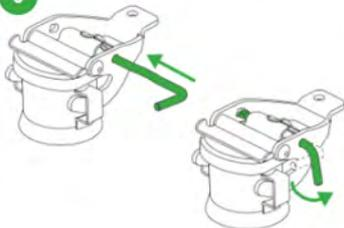
Insert the locking pin through the lever and rotate it 90 degrees.
