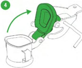
4 By pulling the lever, lift the lid up to open the neck opening.
