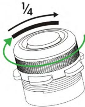
Screw the cap until you feel resistance. Then turn the cap an additional 1/4 of a turn. Do not tighten the cap too much, as it may be difficult to unscrew.
