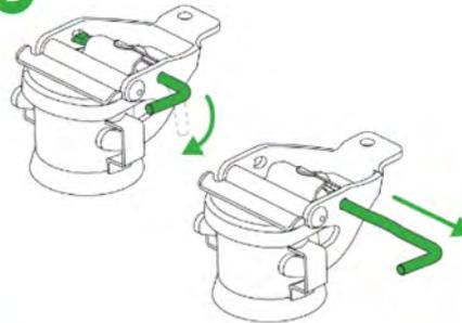
Turn the locking pin and pull it out of the lever as far as it will go.
