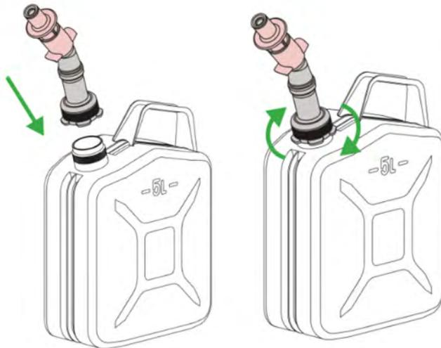
Screw the spout on by turning it clockwise until you feel resistance of the seal. Then turn the spout an additional  $\frac{1}{4}$  of a turn.
