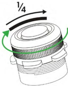
Screw the cap until you feel resistance. Then turn the cap an additional  $\frac{1}{4}$  of a turn. Do not tighten the cap too much, as it may be difficult to unscrew.
