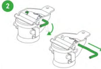
2 Turn the locking pin and pull it out of the lever as far as it will go.
