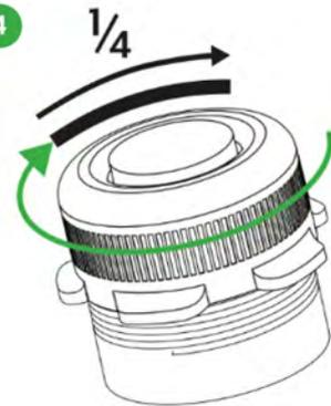
Screw the cap until you feel resistance. Then turn the cap an additional 1/4 of a turn. Do not tighten too much as it may be difficult to unscrew.
